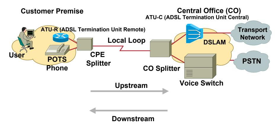
Like Dial, Cable, Wireless, and E1, DSL Is a Transmission Technology
